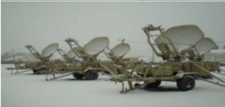
Satellite Terminal Trailer (STT)
